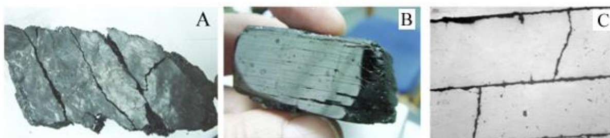
A) in a piece bounded by spalling cracks; B) in a polished block section; C) under a microscope
