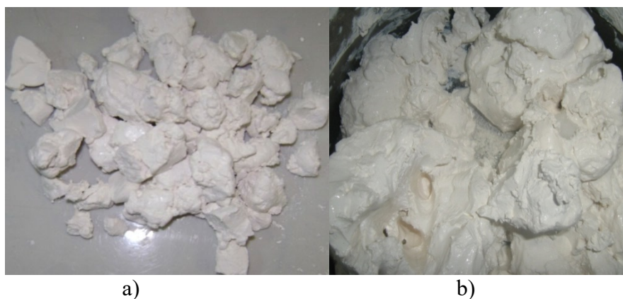
a) titanium dioxide (paste); b) tailings from the enrichment of titanium concentrates
