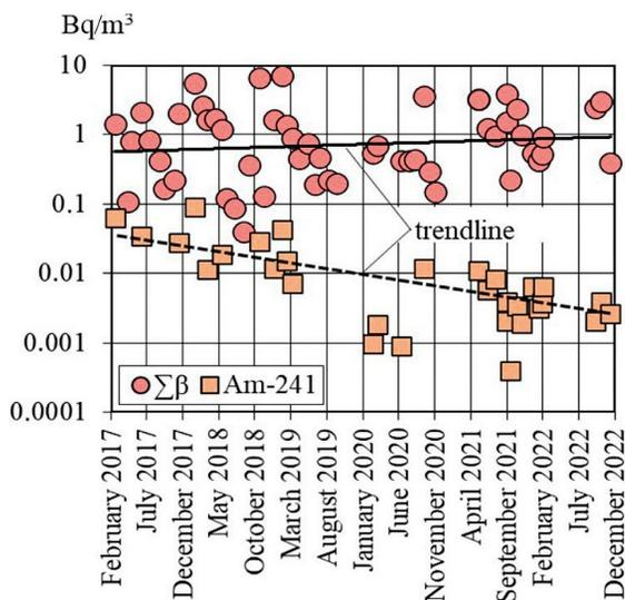
Fig. 2. VA of aerosols carrying  $\Sigma\beta$  and <sup>241</sup>Am in room 012/7 in 2017–2022
