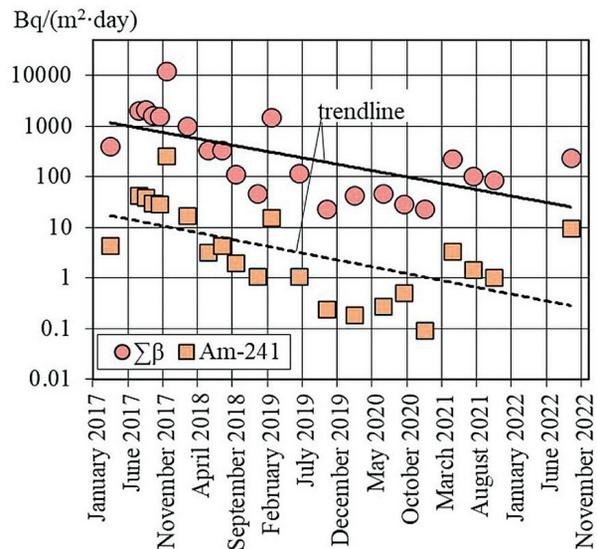
Fig. 3. Deposition density of  $\Sigma\beta$  and <sup>241</sup>Am in room 012/7 in 2017–2022
