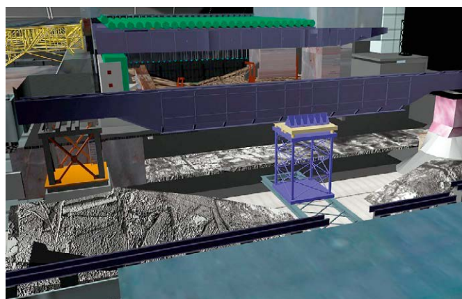
Fig. 16. The middle movable part of the temporary support is moved along the stationary part and set in the design position under the beam
