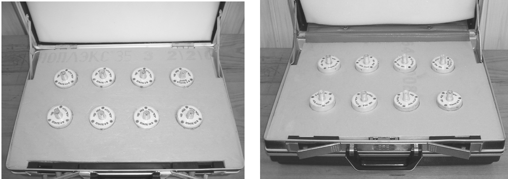
Fig. 14. External view of a complete set of standard (left) and portable (right) thermoelectric voltage converters developed at NTTU "KPI" Research and Development Institute for Experimental Research Automation.
