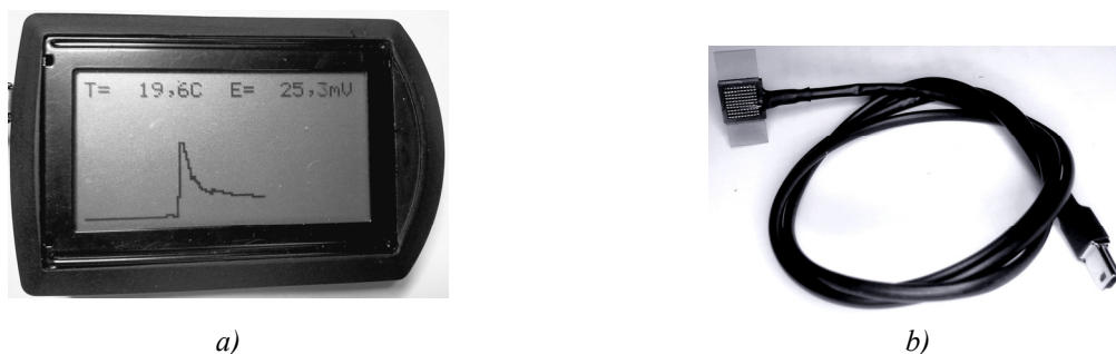
a) measuring unit appearance, b) heat flux thermoelectric sensor appearance.
