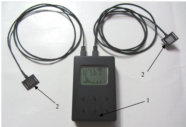
Fig. 1. Modernized device for human heat flux measurement: 1 – electronic recorder, 2 – thermoelectric sensor of heat flux and temperature.
