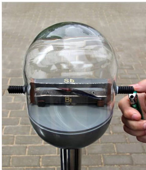
Working model of Seebeck's experiment
