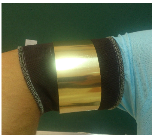
Fig. 1. The appearance of TES for a local thermal effect on human hand.
