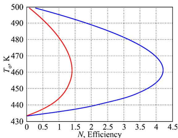
Fig. 9. The ratio between temperature  $T_o$ , power and efficiency of TEG at  $0 \leq m \leq \infty$ .
