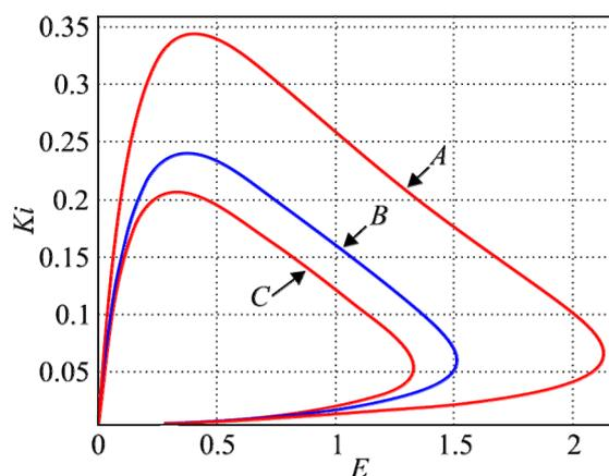
Fig. 13. Comparison of various THP schematics with identical cooling depth ( $T_o = 280$  K).
