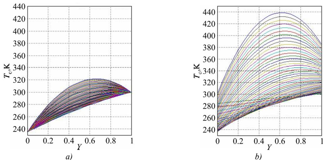
Fig. 1. Temperature distributions in thermoelement, THP mode,  $0 \leq J \leq J_{\max}$ .
