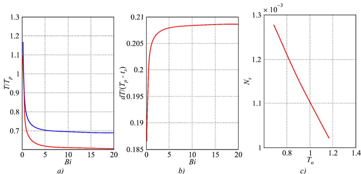
Fig. 10. Characteristics of TEG at  $Ki < Ki_{max}$ : a) – dependence of junction temperatures on  $Bi_h$  ( $- T_o/T_p$ ;  $- T_h/T_p$ ); b) – dependence of relative operating temperature difference  $dT/(T_p - t_x)$  on  $Bi_h$ ; c) – the ratio between the specific power of TEG  $N_s$  and the temperature of the heat-absorbing junction  $T_o/T_p$ .
