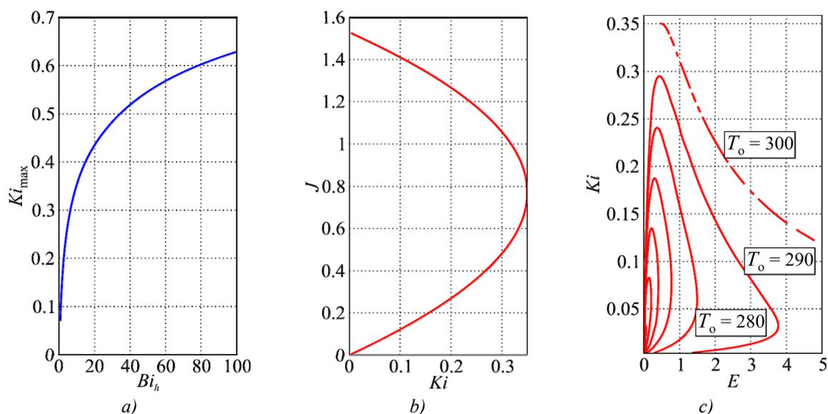
Fig. 7. a) Dependence of maximum possible cooling capacity  $Ki_{max}$  on  $Bi_h$  criterion.
