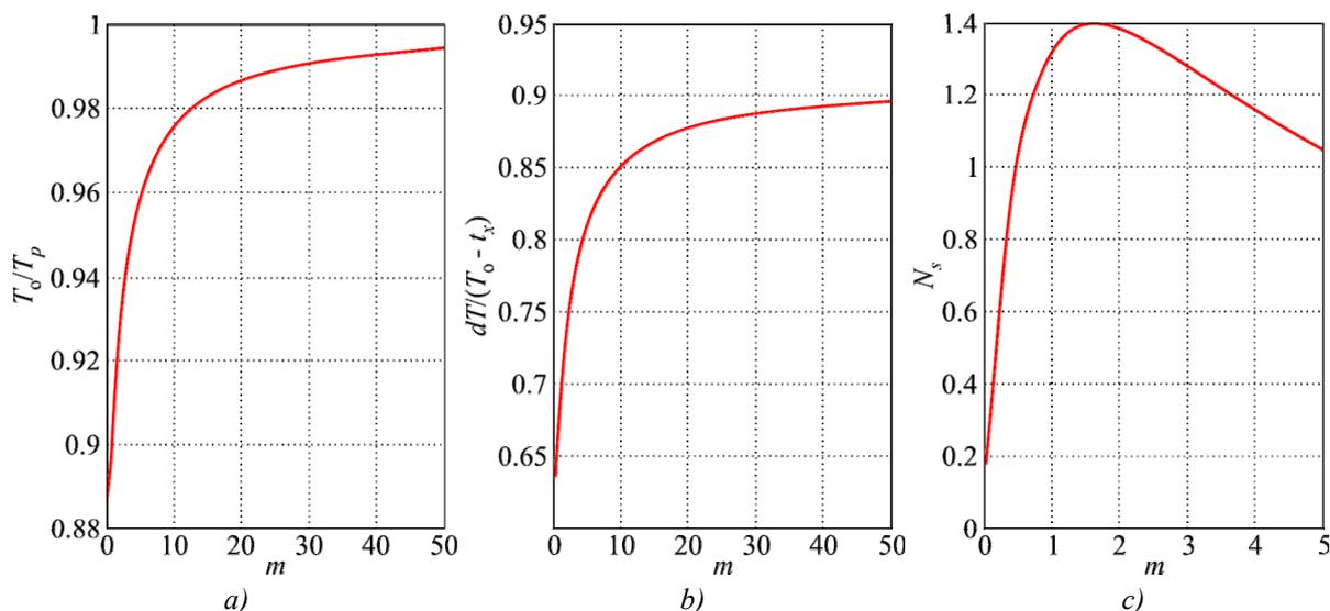
Fig. 8. Effect of load factor on TEG characteristics: a) –dependence of relative temperature of the heat-absorbing junction on  $m$ ; b) – dependence of relative operating temperature difference on  $m$ ; c) – dependence of specific power  $N_s$ ,  $W/cm^2$ , on  $m$ .
