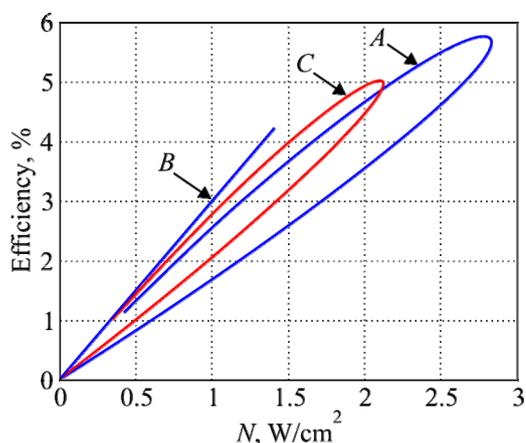
Fig. 12. The ratio between power and efficiency of TEG for different schematics ( $T_p = 500$  K,  $0 \leq m \leq \infty$ )
