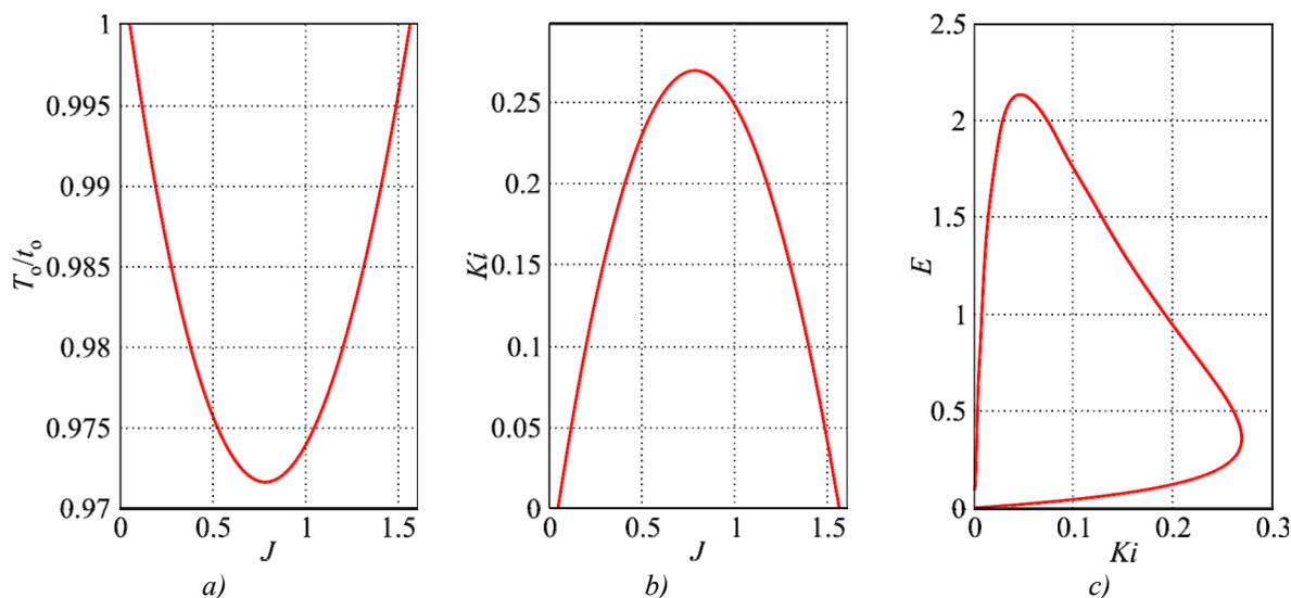
Fig. 11. Characteristics of THP of heat-exchange type: a) – dependence of relative temperature of the heat-absorbing junction ( $T_o/t_o$ ) on  $J$ ; b) – dependence of THP heat capacity on  $J$ ; c) – the ratio between cooling capacity  $Ki$  and THP efficiency  $E$ .
