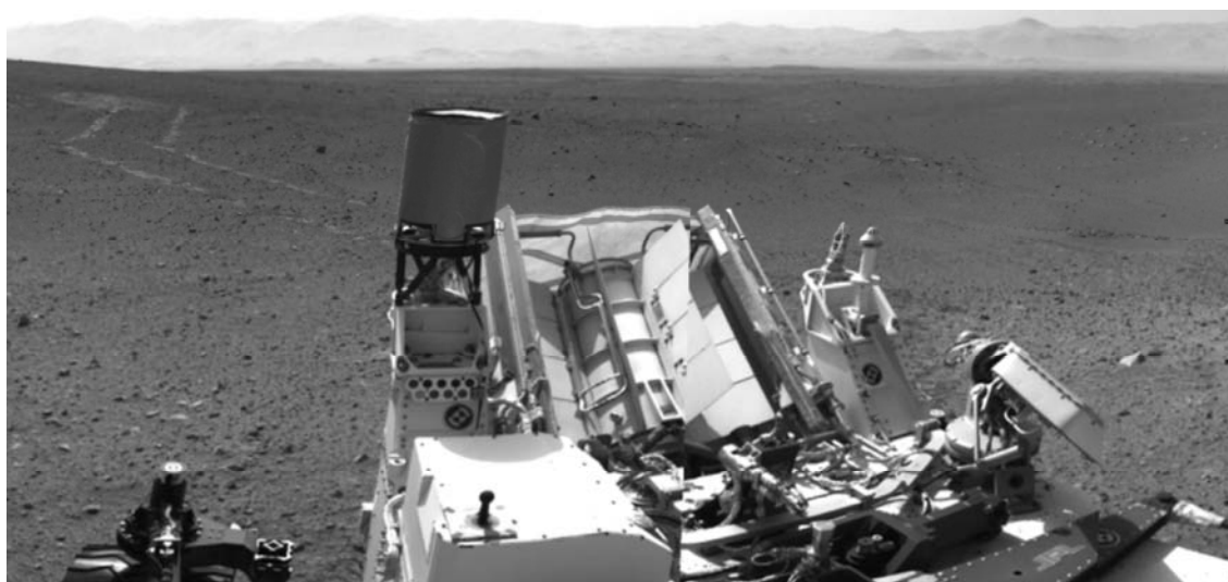
Fig. 2. MMRTG on Mars. This image was taken on sol 24.
