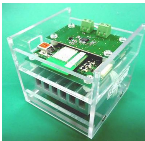
Fig. 9. Commercial proto-type TEPG-integrated wireless sensor node device.
