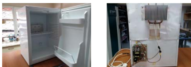
Fig. 7. Joint project of TÜBİTAK and company TES Ltd “Thermoelectric minibar with a heat pipe”.
