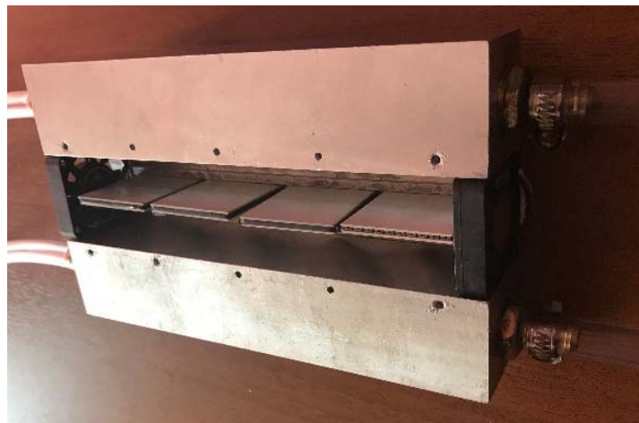
Fig. 2. Appearance of thermoelectric heat transfer intensifier
