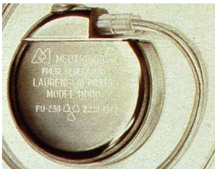
Fig. 12. Cardiac pacemaker with a radioisotope thermoelectric generator [53]
