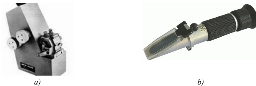
Fig. 2. Refractometers: a) laboratory IRF 454B2 M b) pocket VBC4T.
