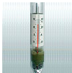
Fig.1. Hydrometer AEF / tosol cooling fluid, antifreeze.
