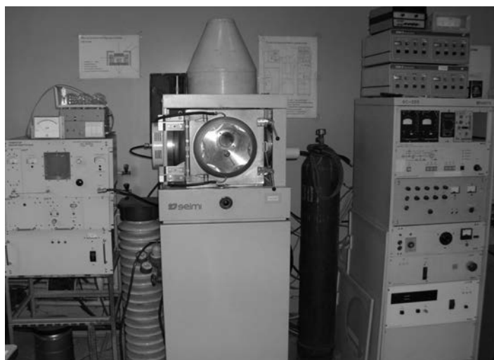
Fig. 1. Installation of high-frequency magnetron sputtering
