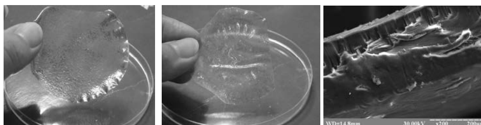
Fig. 2. Chitosan films with different types of copper coatings and electron microscopy of the film cross section
