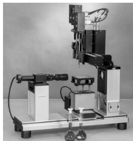
Fig. 7. Optical contact angle measuring and contour analysis systems OCA-50EC (Dataphysics Instruments, GmbH, Germany)
