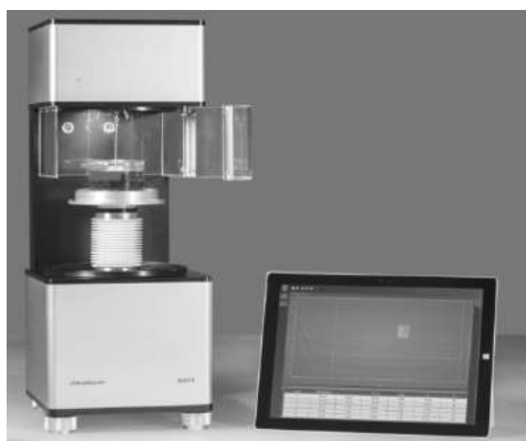
Fig. 5. Dynamic Contact Angle measuring device and Tensiometer DCAT-9 (DataPhysics Instruments GmbH, Germany)
