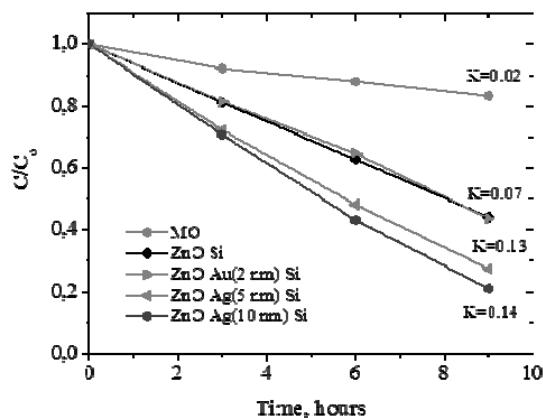
**Fig. 5.** Kinetics of MO dye photodegradation by the help of ZnO, ZnO/Ag and ZnO/Au NS deposited on Si wafers under illumination with 200 W Hg lamp
