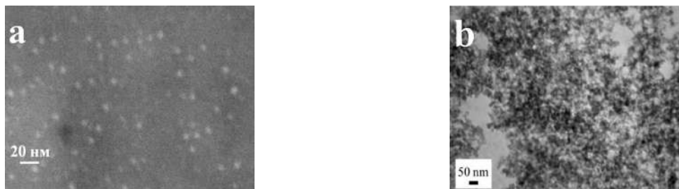
Fig. 4. a – SEM image of Ag 2 %/SiO 2 film, b – SEM image of dispersed Ag(0.0016 %)/SiO 2 [13]
