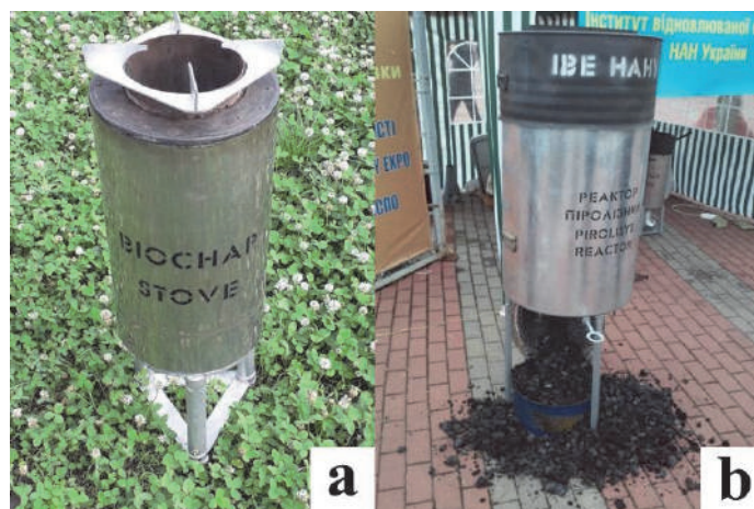
Fig. 1. (a) Household portable and (b) farmer's stoves for oxidative pyrolysis of biomass, adapted from [64, 65]
