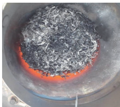
Fig. 2. Visualization of chips heating and charring in the stove reactor
