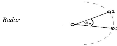
FIG. 4. Location of targets and radar when determining resolution along azimuth
