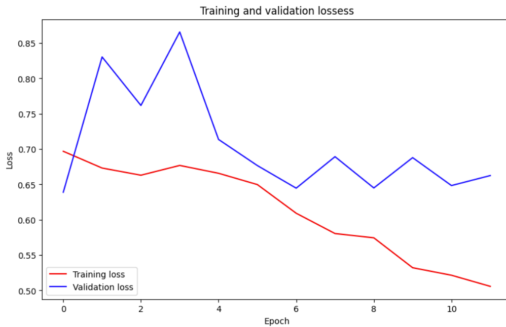
FIG. 1. Loss of the model per training epoch. Red line corresponds to training data, blue to validation data
