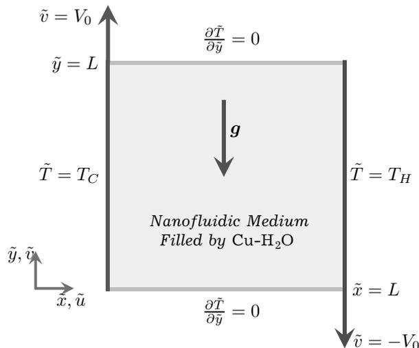
**Fig. 1.** Geometrical configuration of the present convective nanofluid flow problem.
