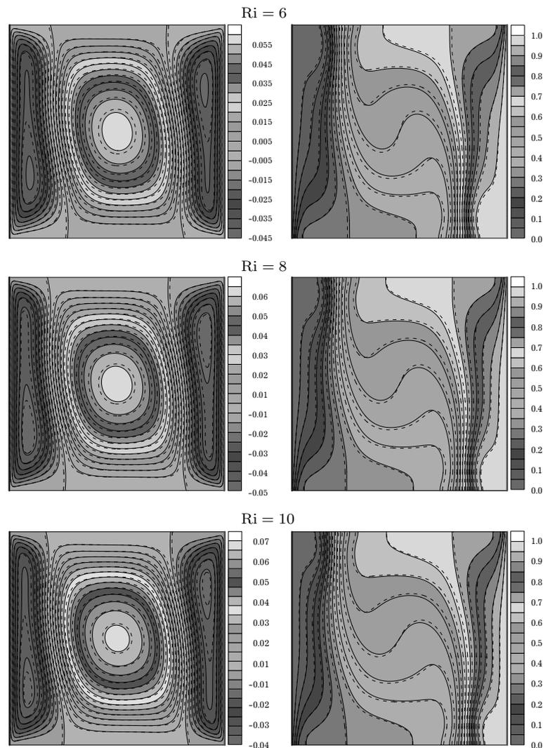
**Fig. 3.** Streamline shapes (left) and isotherm contours (right) of water (dashed line) and copper-water nanofluid (solid line) for various values of  $Ri$ , when  $\chi = 0.01$  and  $d_{np} = 30$  nm.
