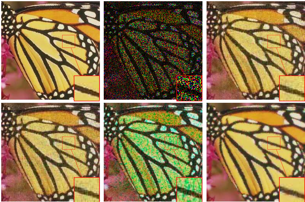
Fig. 3. The visual comparison results of the recovered Image 1 . The original image, the incomplete image with 30% of observation, the recovered results by TNNR, LRTC, MFTV, and the proposed NCTV respectively.
