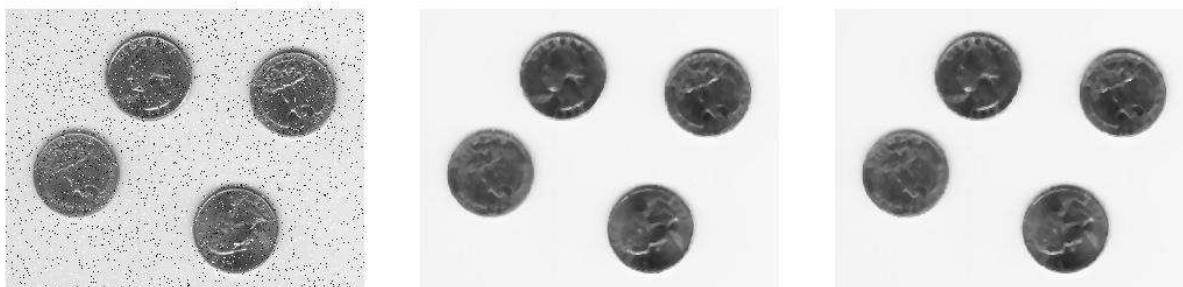
Fig. 7. Left: Noisy image by salt and pepper noise, restored image obtained by the proposed model. Middle: D2Q5 model. Right: D2Q9 model.
