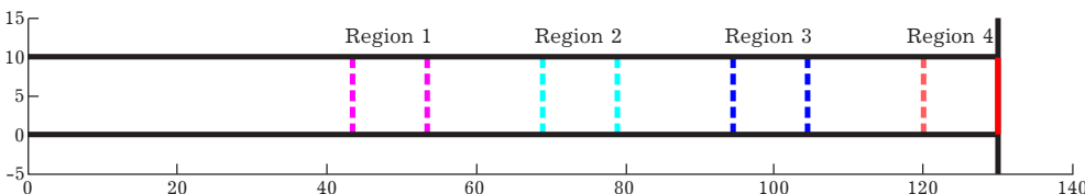
Fig. 1. Geometry of the simulated domain. The gate is placed on the far right. Pedestrian density evolution is monitored within the four square regions placed along the corridor.
