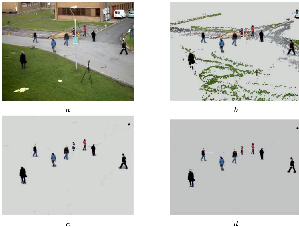
Fig. 3. The background subtraction result on PETS2009-View001 [39].
