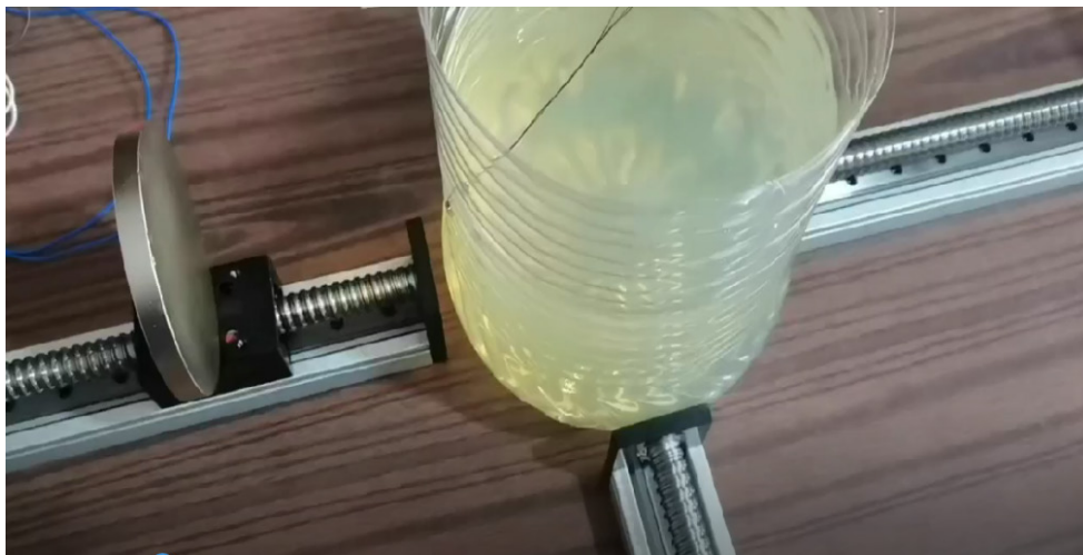
Figure 13 – When large permanent magnets move away, small permanent magnets stay at the boundary position.
