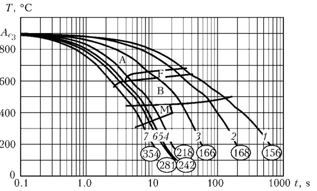
**Figure 1.** CCT diagram of austenite transformation of 10G2FB steel: 1 –  $w_{6/5} = 1.5$ ; 2 – 3; 3 – 10; 4 – 30; 5 – 38; 6 – 45; 7 –  $55 \text{ }^\circ\text{C/s}$ ; A – austenite; B – bainite; F – ferrite; M – martensite; figures in circles – Vickers hardness
