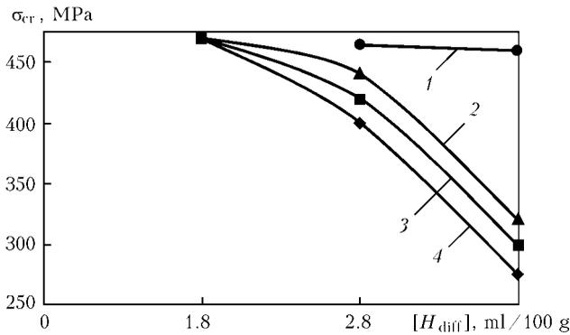
**Figure 5.** Dependence of critical stresses on concentration of the diffusion hydrogen and cooling conditions of the HAZ metal during testing by Implant method with preheating to 90 (1), 60 (2), 40 (3) °C and without preheating (4)
