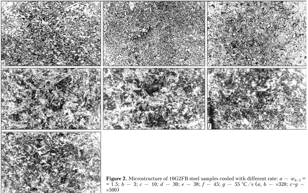
**Figure 2.** Microstructure of 10G2FB steel samples cooled with different rate: a –  $w_{6/5} = 1.5$ ; b – 3; c – 10; d – 30; e – 38; f – 45; g –  $55 \text{ }^\circ\text{C/s}$  (a, b –  $\times 320$ ; c–g –  $\times 500$ )
