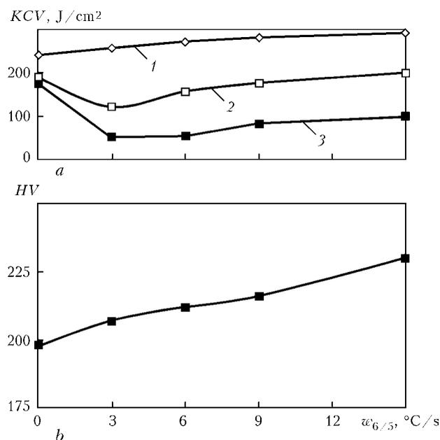
Figure 4. Influence of cooling rate on impact toughness (1 – +20; 2 – -20; 3 – -40 °C) (a) and hardness (b) of overheating area of the HAZ metal
