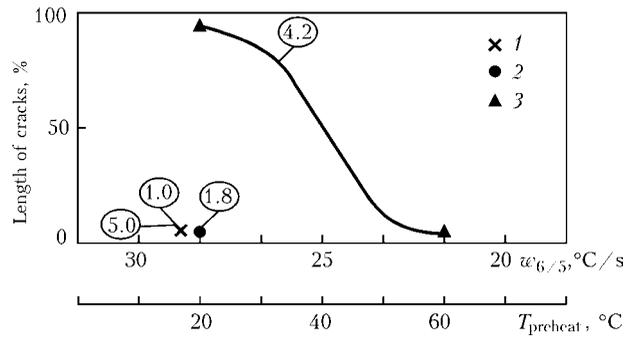
**Figure 6.** Influence of cooling rate  $w_{6/5}$ , preheating temperature  $T_{preheat}$  and diffusion hydrogen content (figure in circles) on length of cracks in 10G2FB steel joints («rigid T-joint» sample): 1 – flux-cored wire Megafil 821R in CO<sub>2</sub> welding; 2, 3 – ANP-10 electrodes
