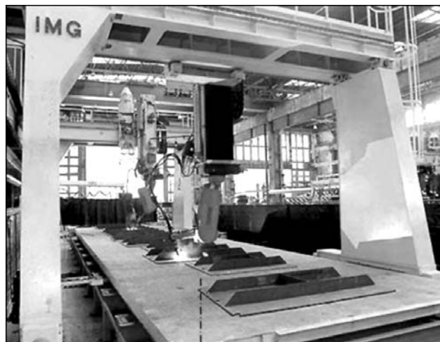
Figure 2. Welding station in micropanel line using two robots before refitting
