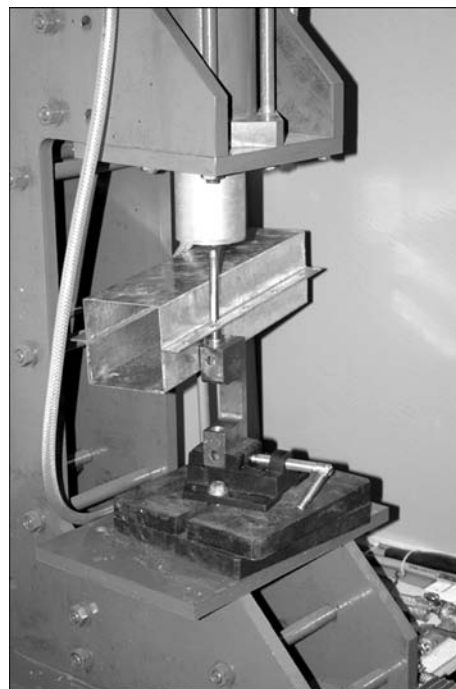
Figure 7. Appearance of pneumatic press for formation of mechanical joints
