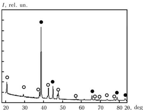
**Figure 4.** Spectrum of X-ray diffraction of rapidly solidified strip of Al + 33 % Cu: ● – Al; ○ –  $\text{Al}_2\text{Cu}$
