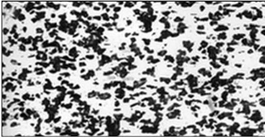
**Figure 1.** Microstructure ( $\times 400$ ) of the AMg5 + 27 %  $\text{Al}_2\text{O}_3$  CM in the initial state
