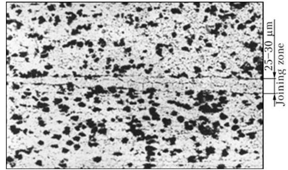
**Figure 5.** Microstructure ( $\times 300$ ) of the CM joining zone in vacuum pressure welding using rapidly solidified strip (Al + 33 % Cu) 0.07 mm thick under free deformation conditions
