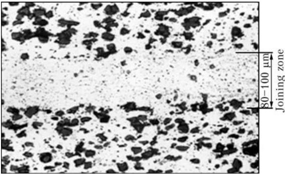
**Figure 3.** Microstructure ( $\times 400$ ) of CM welded joint produced by vacuum pressure welding using aluminum interlayer 0.15 mm thick under forced deformation conditions
