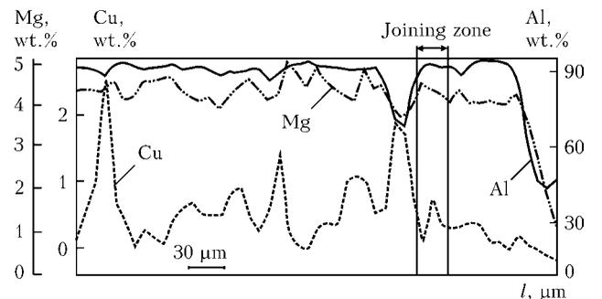
**Figure 6.** Character of distribution of copper, magnesium and aluminum in the CM joining zone in welding under free deformation conditions
