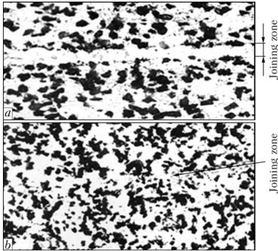
**Figure 7.** Microstructure of the CM joining zone ( $\delta = 8\text{--}10\ \mu\text{m}$ ) in vacuum pressure welding using rapidly solidified strip (Al + 33 % Cu) under forced deformation conditions (*a* –  $\times 600$ ) and with subsequent thermal cycling (*b* –  $\times 400$ )
