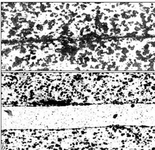
**Figure 2.** Microstructure of the welded joint on AMg5 + 27 %  $\text{Al}_2\text{O}_3$  CM produced by vacuum pressure welding without interlayer (*a* –  $\times 400$ ) and with aluminum interlayer 0.15 mm thick under free deformation conditions (*b* –  $\times 250$ )
