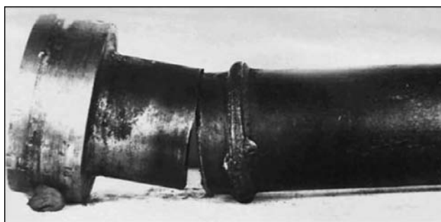
Figure 11. Part of torque rod after cyclic tests
