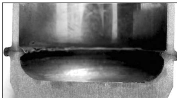
Figure 8. Macrosection ( \times 1.5 ) of welded joint of shock-absorber
