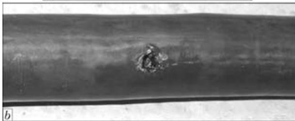
**Figure 1.** High-voltage insulator of high alumina ceramics (a) and high-voltage cable (b), withstood the test voltage of 120 kV but destroyed in the process of operation of standard power unit ELA-60 (rated voltage of 60 kV)
