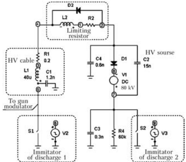
**Figure 3.** Diagram for modeling transition processes (for designations see the text)
