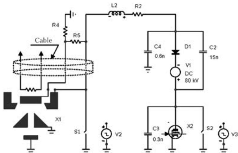
**Figure 2.** Simplified schematic diagram of standard power unit ELA-60 with elements for modeling transition processes (for explanations see the text)
