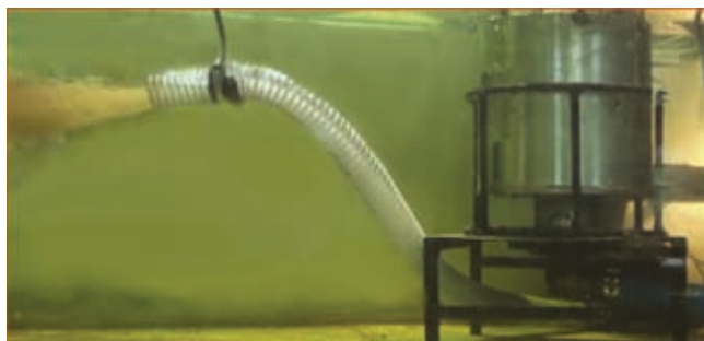
Connection of the module to the emergency well for further transportation of fluid via the pipeline
