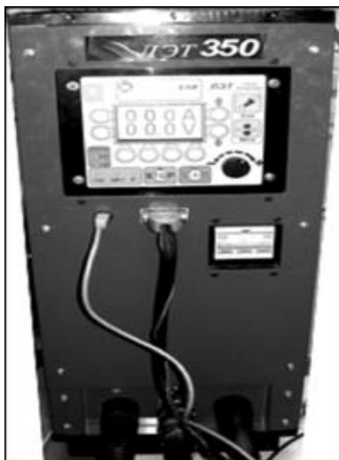
Figure 2. Variant of design of welding current source LET 350 with metallic sheath and touch-type display
