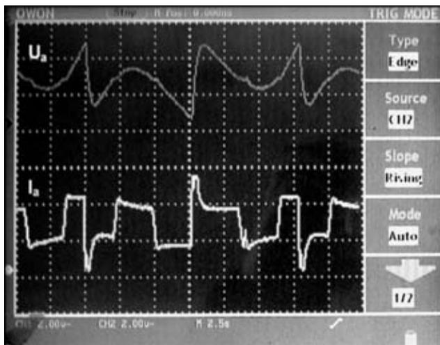
Figure 4. Oscillograms of armature voltage  $U_a$  and current  $I_a$  of motor of the additional drive at execution of triangular trajectory of the electrode movement
