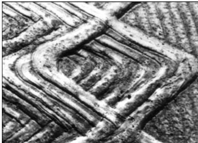
**Figure 1.** Surface of the roll with deposited zigzag-shape beads
