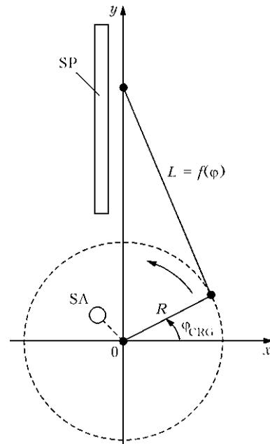
Figure 2. Kinematic scheme of the drive: SA – sensor of crank rotation angle; SP – sensor of electrode position
