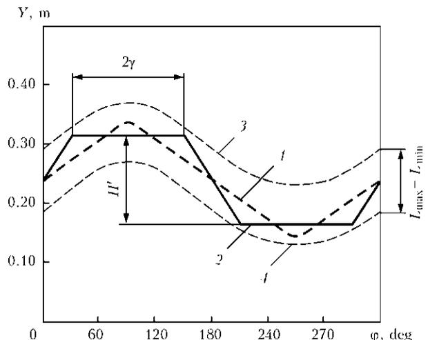
Figure 3. CRG trajectories: 1 – triangle; 2 – trapezoidal; 3, 4 – with proposed  $L_{max}$  and  $L_{min}$ , respectively
