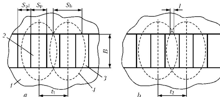
Figure 6. Scheme of groove and expected penetration shape in MESW with consumable nozzle:  $a - l = 0$ ;  $b - l > 0$ ; 1 – body of workpiece subject to repair; 2 – filled-in hole; 3 – shaping spacer plate; 4 – isotherm of melting;  $t_1$  and  $t_2$  – distances between axes of filled-in holes (pitch)
