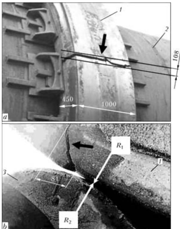
**Figure 1.** Through cracks in bands of rotary cement kilns 5 m in diameter: *a* – deviation of crack from the cross section plane of the band; *b* – deviation from the radial plane; 1 – band; 2 – kiln casing; 3 – bearing roller;  $R_1 = 3050 \text{ mm}$  – radius of roll surface of band;  $R_2 = 450 \text{ mm}$  – radius of bearing roller
