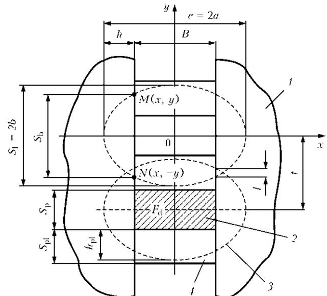
Figure 3. Scheme for calculation of groove and penetration shape in MESW: 1 – body of workpiece subject to repair; 2 – filled-in hole; 3 – penetration shape; 4 – bridge;  $e$  – width of a layer of multilayer weld;  $S_{pl}$  – thickness of shaping spacer plate;  $S_1$  – thickness of a layer of multilayer weld (see the text for the rest of the designations)
