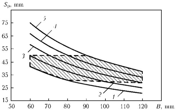
Figure 2. Range of optimal ratios of gap width  $B$  to pit width  $S_p$  for MESW with twin-electrode consumable nozzle: 1 –  $F_d = 2500$ ; 2 – 3000; 3 – 3500; 4 – 4000; 5 – 4500 mm<sup>2</sup>
