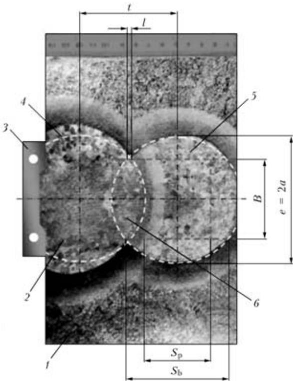
**Figure 7.** Transverse macrosection of a fragment of multilayer electroslag weld: 1 – workpieces welded; 2 – shape of groove for MESW; 3 – water-cooled shaping device; 4 – calculated shape of fusion line (zone); 5 – weld layer; 6 – shaping spacer plate
