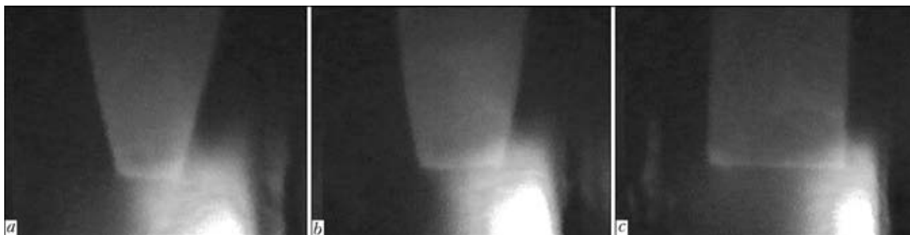
Figure 4. Photos (light filter IKS-5) of the 5 mm diameter flat-tip electrode with a tip width of 1 ( a ), 2 ( b ) and 5 ( c ) mm, and the arc gap in narrow-gap welding at I_w = 400 A
