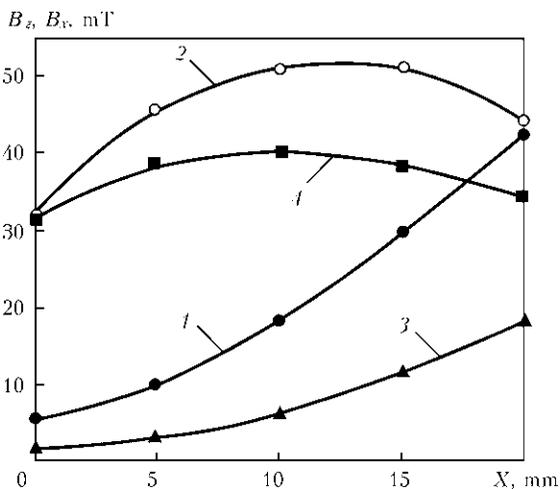
**Figure 2.** Distribution of components of induction  $B_z$  and  $B_x$  of TMF along the axis OX ( $Z = 0, Y = 0, I_{\text{coil}} = 60$  A): 1, 3 —  $B_z$ ; 2, 4 —  $B_x$ ; 1, 2 — constant TMF; 3, 4 — alternating TMF of 50 Hz frequency
