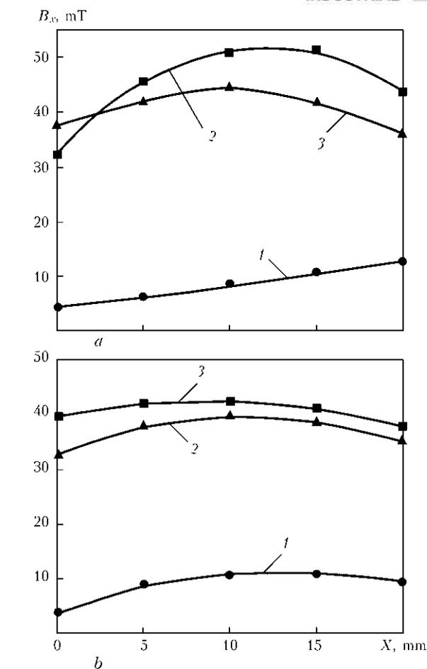
**Figure 3.** Distribution of induction  $B_x$  of constant (*a*) and alternating TMF of 50 Hz frequency (*b*) along the axis  $OX$  depending on ferromagnetic properties of welding wire of 4 mm diameter and base metal ( $Z = 0$ ,  $Y = 0$ ,  $I_{\text{coil}} = 60$  A): 1, 2 – wire Sv-08GA; 3 – Sv-12Kh18N10T; 1 – plate 09G2S; 2, 3 – 12Kh18N10T
