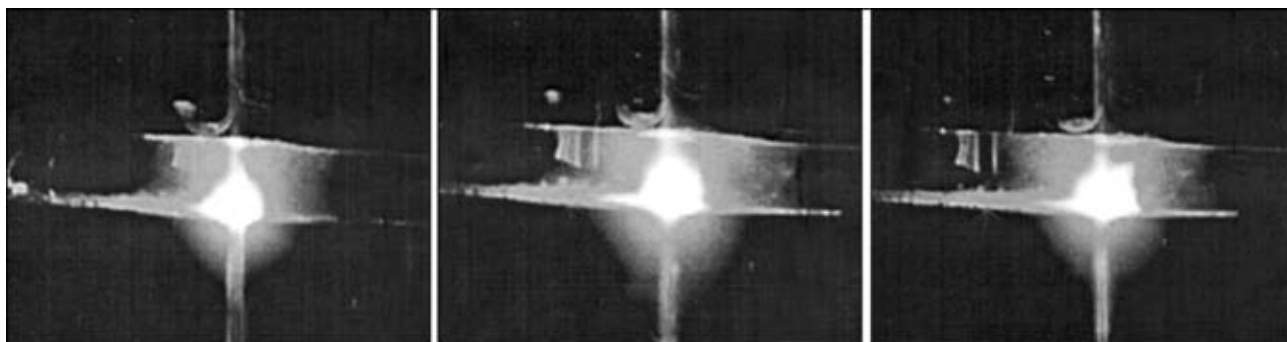
Figure 7. Three successive fragments of arcing phases in electric submerged-arc welding obtained in an experiment (see Figure 6) when welding process runs from left to right
