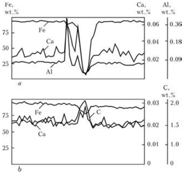
**Figure 3.** Distribution of main alloying elements Ca, Al (a) and Ca, C (b) in deposited metal produced by using flux-cored wire PP-Np-Op-3
