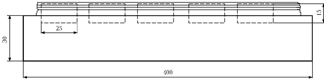
Figure 1. Scheme of cutting out of specimens for tribotechnical investigations of deposited metal
