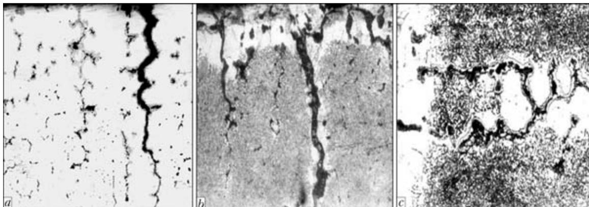
**Figure 2.** Microstructures of deposited metal produced by using the flux-cored wire PP-Np-Op-3: *a* – section without etching (surface layer),  $\times 250$ ; *b* – the same with etching in nitric acid,  $\times 200$ ; *c* – central zone of specimen section with etching in nitric acid,  $\times 500$
