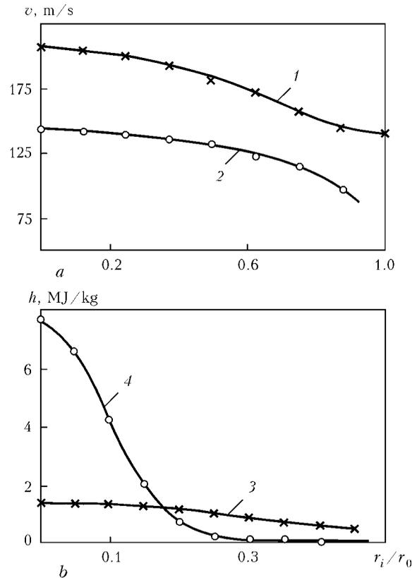
**Figure 2.** Distribution of speed (a) and enthalpy (b) of particles on radius of spraying spot in application of tip (1, 3) and without it (2, 4) [13]
