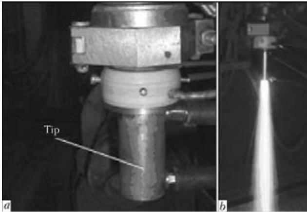
Figure 7. Appearance of tip (a) and spraying jet (b) with application of PT-NA-01 powder
