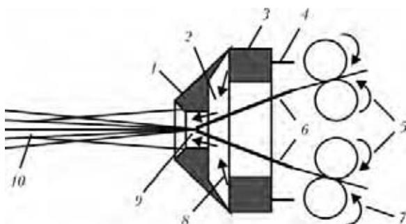
**Figure 1.** Scheme of activating electric arc metallizing [8]: 1 – nozzle; 2 – collector; 3 – combustion chamber; 4 – mixture of air with combustible gas; 5 – feeder; 6 – guides; 7 – wires; 8 – spraying gas; 9 – arc; 10 – jet
