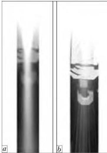
**Figure 3.** Appearance of plasma jet in spraying of metallic (a) and ceramic (b) powders
