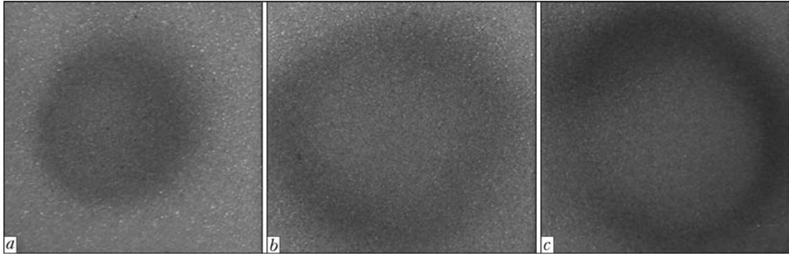
Figure 6. Spraying spot in coating with application of tip (a), cylinder part of tip (b) and without it (c)
