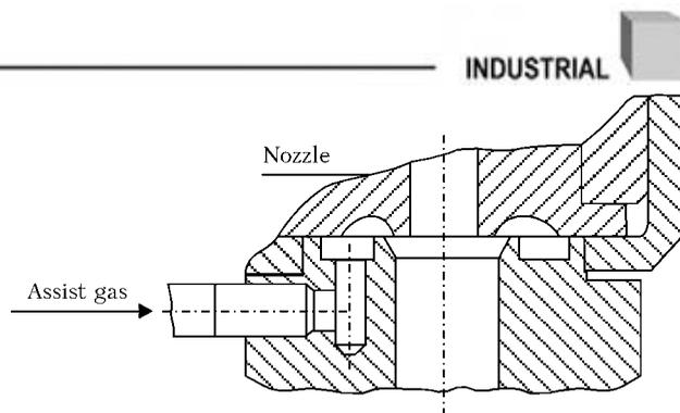
**Figure 4.** Scheme of feed of assist gas in a tip
