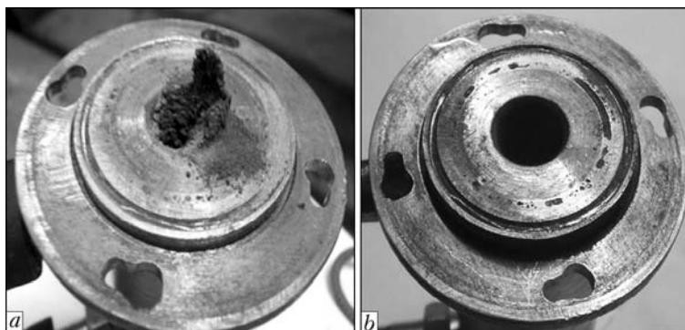
**Figure 4.** Appearance of lower part of tip after spraying at consumption of transporting gas  $0.360$  (a) and  $0.264$  (b)  $\text{m}^3/\text{h}$
