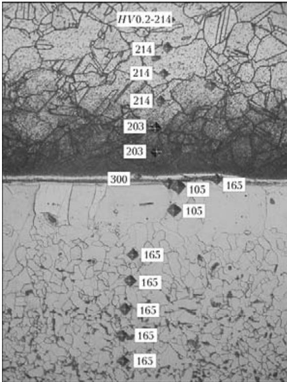
**Figure 2.** Microstructure ( $\times 100$ ) of bimetal in the section of transition from boiler pearlitic steel (*below*) to austenitic cladding layer (*above*)
