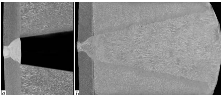
**Figure 5.** Weld macrostructure in the cladding layer (*a*) made in the welded joint of clad pipe steel by the developed technology (*b*)
