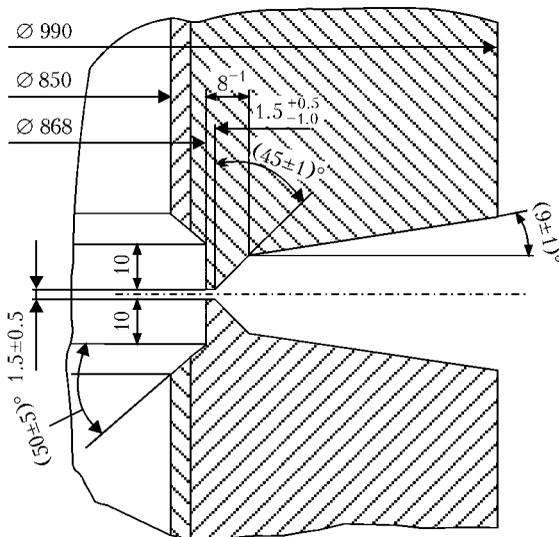
**Figure 1.** Schematic of edge preparation of pipe butt joint from clad steel welded by the standard technology
