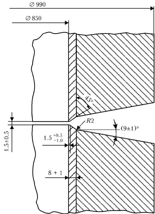
**Figure 3.** Schematic of edge preparation for welding from one side of pipe joint from clad low-alloyed steel
