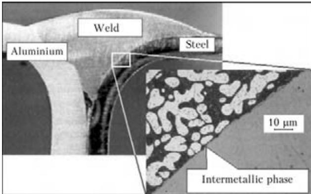
**Figure 3.** Schematic of laser braze-welding in car manufacture [23]
