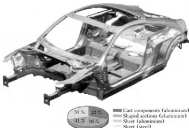
Figure 1. Structure of Audi TT body from dissimilar materials [4]
