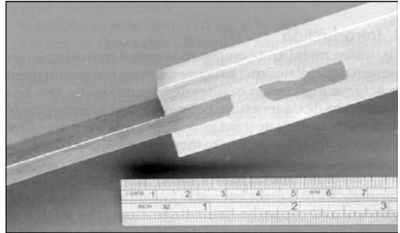
**Figure 7.** Locking a perforated steel sheet in the aluminium one by stir-lock process
