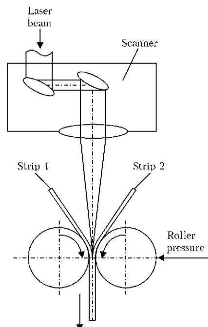
**Figure 5.** Schematic of laser-press welding
