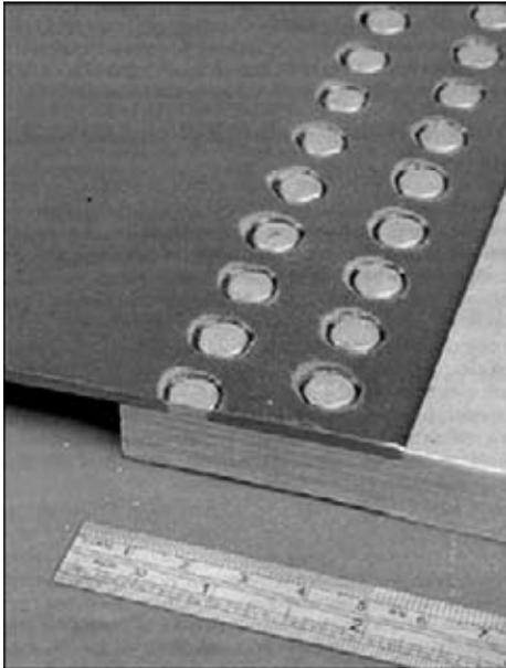
**Figure 6.** Example of joining steel and aluminium sheets by stir-lock process
