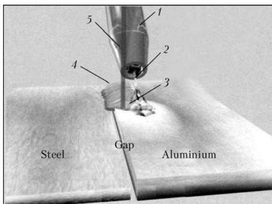
**Figure 4.** Schematic of hybrid laser-arc welding [17]: 1 – welding torch; 2 – filler wire; 3 – weld pool; 4 – weld; 5 – laser beam
