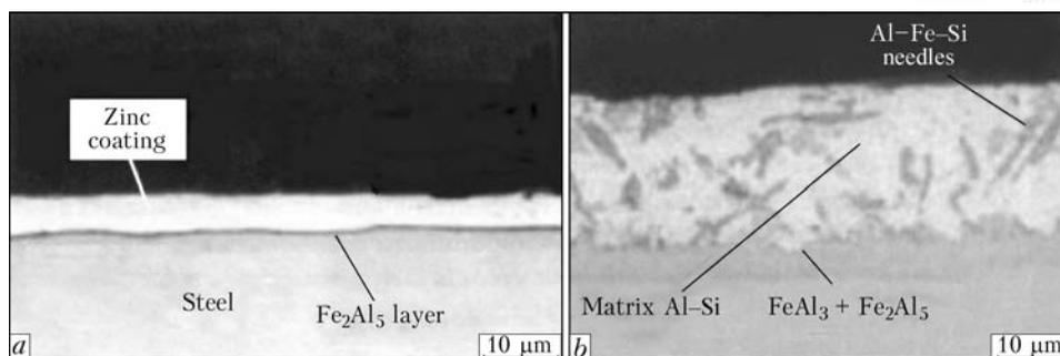
**Figure 2.** Microstructures of joints of aluminium to steel with zinc (a) and aluminosilicate (b) coatings
