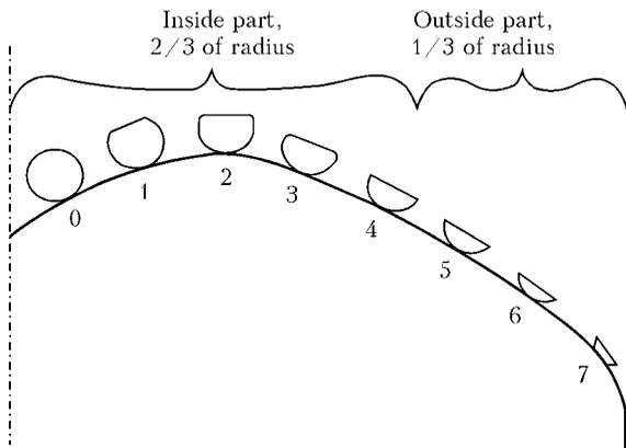
**Figure 1.** Schematic of wear of cutting structure
