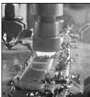
Process of coating using FSS method
