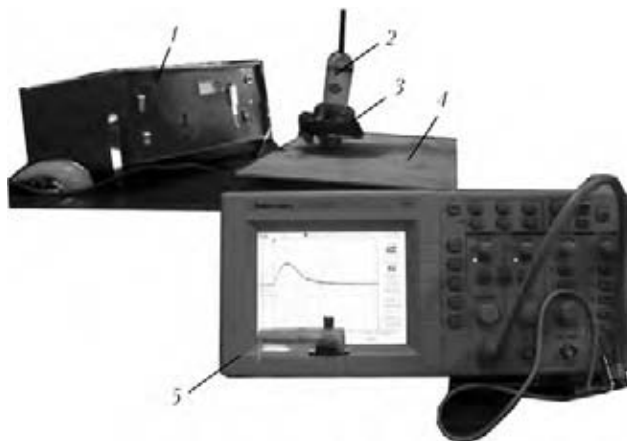
Figure 5. GFI-1 system for measurement of pulsed MF intensity at EDT: 1 – power source for EDT; 2 – Hall sensor; 3 – flat inductor; 4 – welded joint sample; 5 – MF intensity recorder
