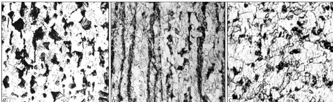
Figure 2. Microstructures ( \times 500 ) of studied steels: a – 15KhSATYuD; b – 10G2FB; c – 06GBD
